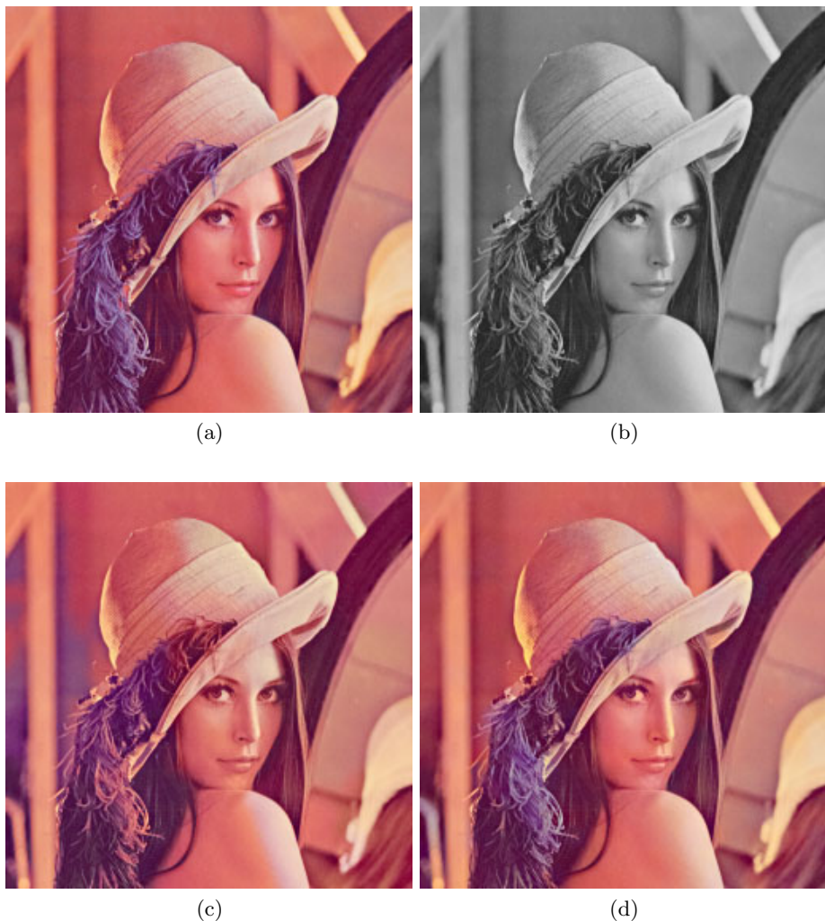
Fig. 1. Experimental results for Lena: (a) original color image, (b) monochrome image, (c) estimated color image using 5 \times 5 references, (d) estimated color image using 20 \times 20 references
