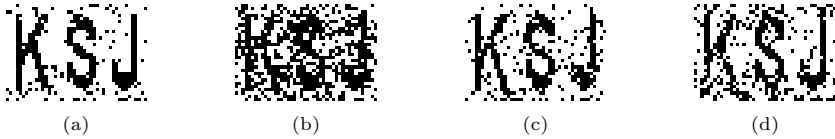
Fig. 9. Watermark images extracted from the FOOTBALL video sequence after various attacks such as (a) spatial LPF, (b) frame dropping, (c) frame average, and (d) MPEG coding
