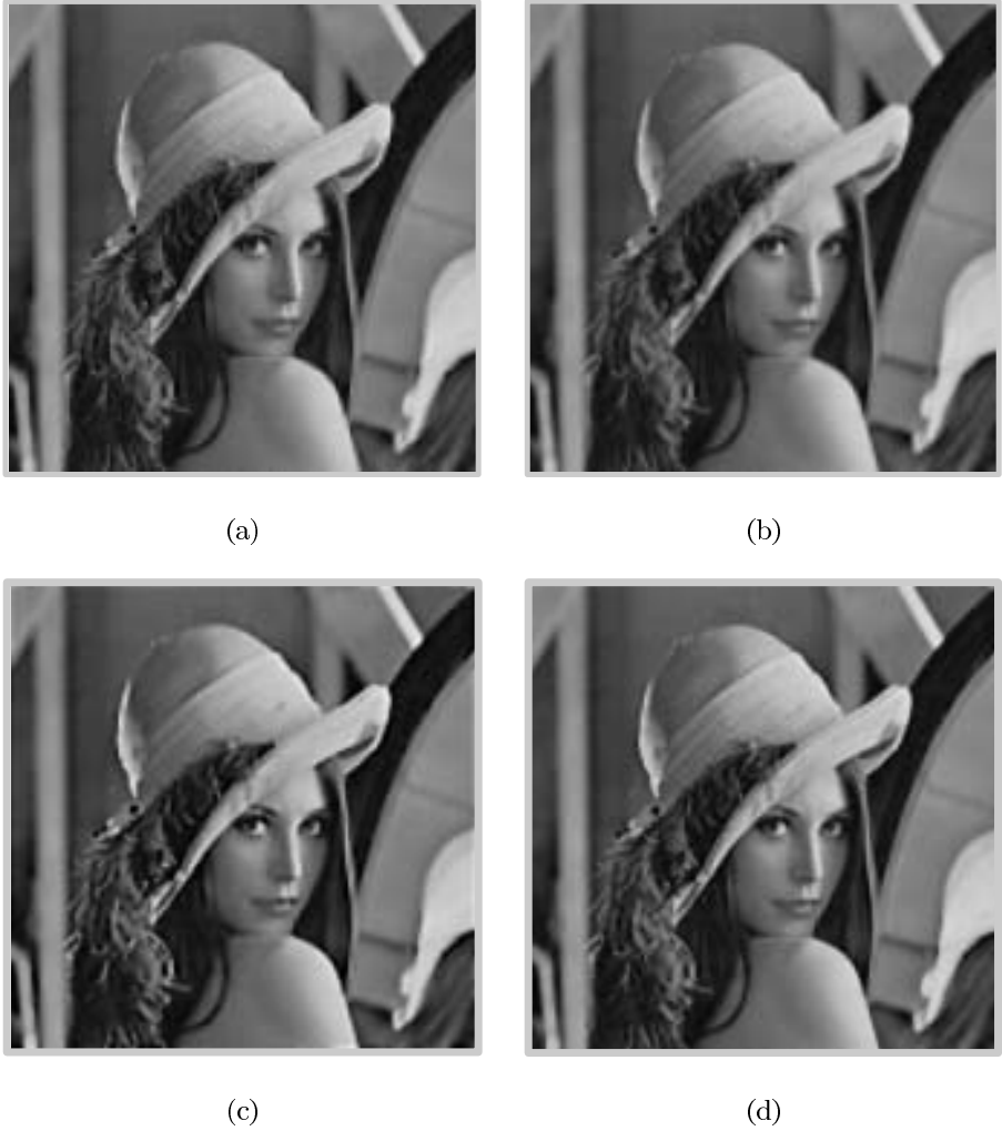
Fig. 3. 256 \times 256 dimensional reconstructed high-resolution results of Fig. 2-a: (a) Zero-order hold interpolation, (b) bilinear interpolation, (c) MAP estimation, (d) proposed algorithm
