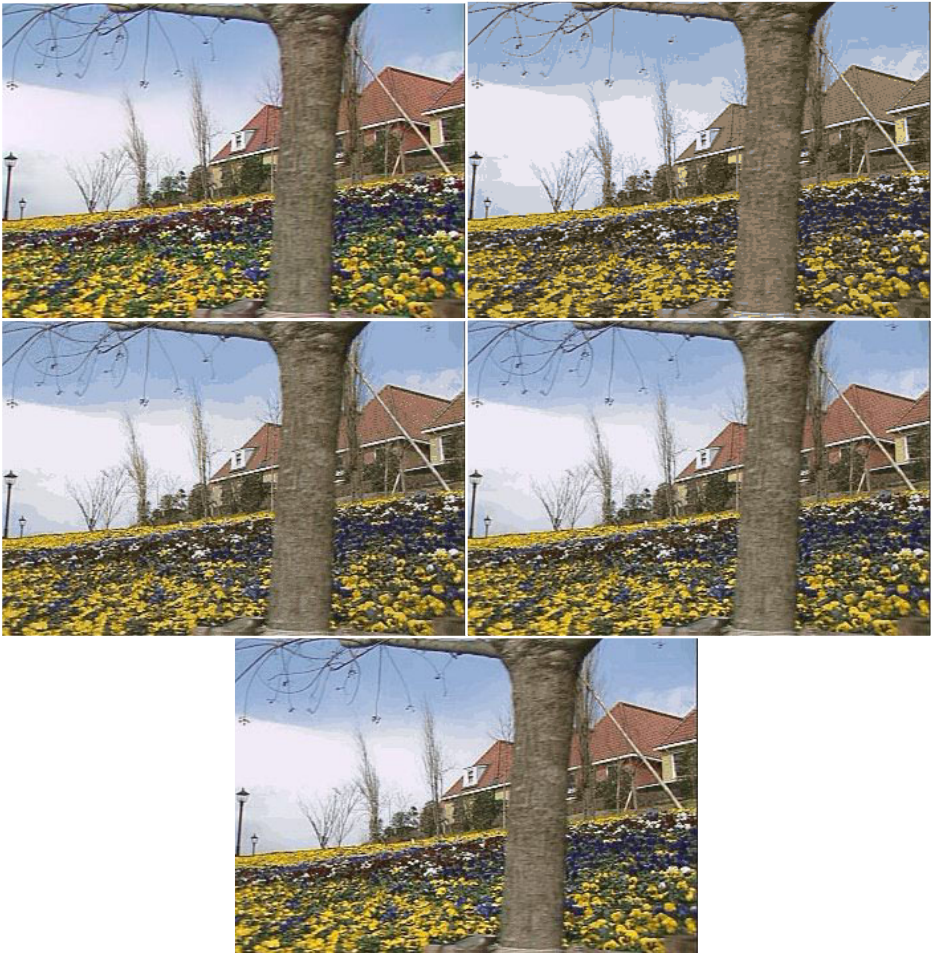
Fig. 2. Quantization results on the image "Garden" are given here. From left to right and top to bottom are the original input image and the quantized ones correspond to quantization level K=16 , K=32 , K=64 , and K=128 respectively. The MSE values are 457, 263, 151, 94.
