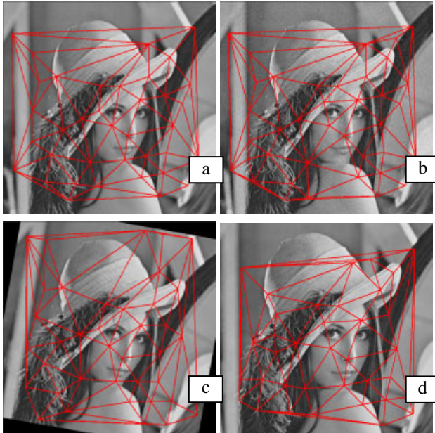
Fig. 2. Patches for watermarking against attacks: (a) original image, (b) image with additive uniform noise, (c) image with rotation 10^\circ , and (d) image with scaling 1.1x
